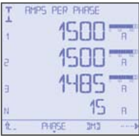
3-phase and neutral current display
