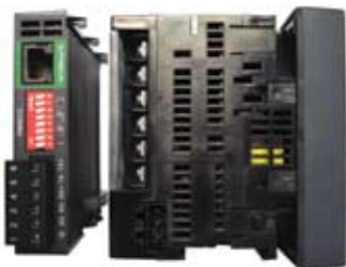
Bottom view of PM8ECC Ethernet communications module and main meter unit, showing Ethernet and RS-485 communication port connectors and configuration switches.
