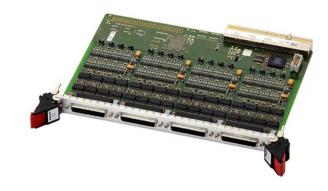
The D302 is an input/output CompactPCI® target board for 128 binary process signals. The I/Os are divided into four optically isolated units. The card is used for input/output of digital signals with different voltage levels and ground references. For each unit 32 channels are driven to the 44-pin D-Sub connector. Each channel can be either input or output.
