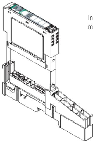
Insert the module straight down into the mounting base.
