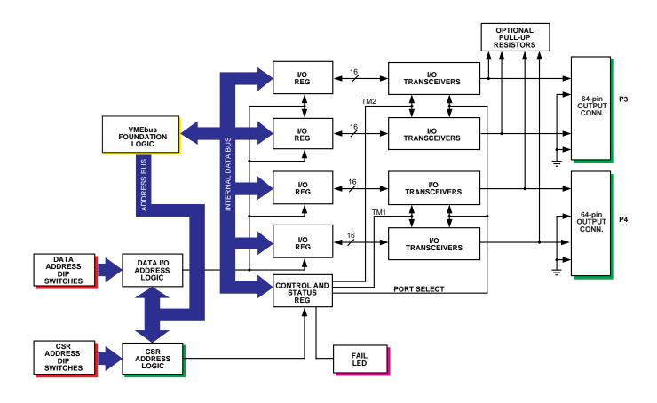
Figure 1. VMIVME-2510B Functional Block Diagram
