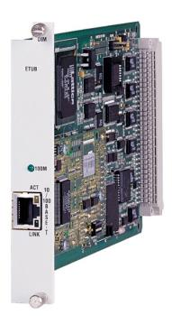
Splits a single high-rate logical channel into up to eight E1/T1 links
