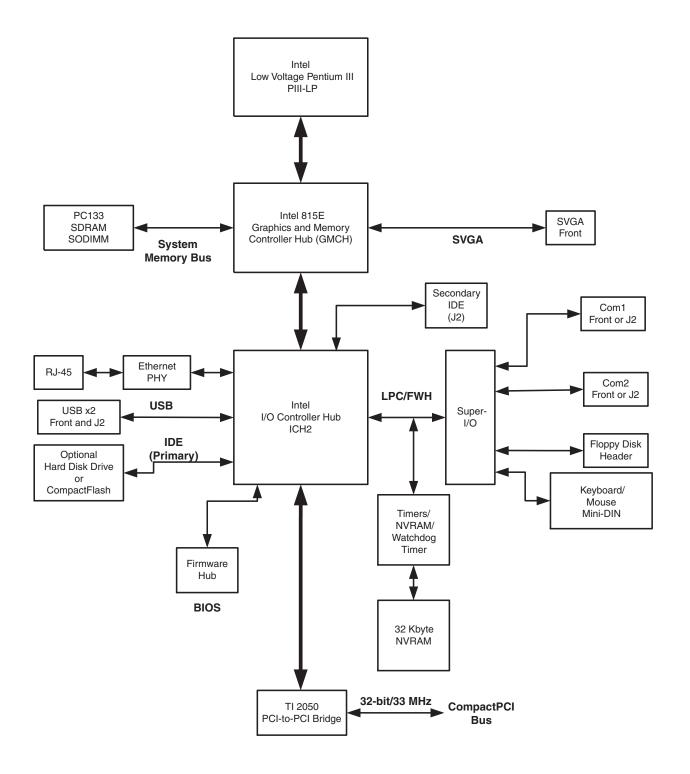
Figure 1. VMICPCI-7505 Low Voltage Pentium III Processor-Based 3U CompactPCI Single-Board Computer
