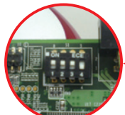
The ID is programmed by a 4-digit DIP switch
