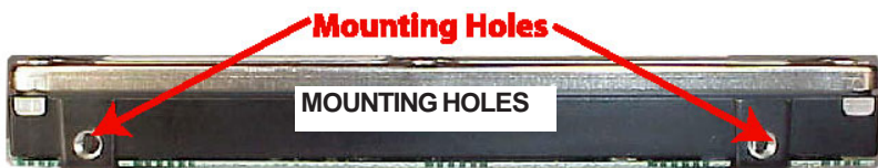
FIGURE 2 – MOUNTING HOLE LOCATIONS
