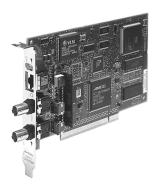
The ControlNet network is an open, state-of-the-art control network that meets the demands of real-time, high-throughput applications. The ControlNet network uses the proven Common Industrial Protocol (CIP) to combine the functionality of an I/O network and a peer-to-peer network providing high-speed performance for both functions.
