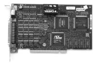
The 1784-PM02AE analog motion card is a 2-axis, closed-loop servo module that you use with a SoftLogix controller. The motion card installs in a 32-bit, local PCI bus slot. You can install as many as four analog motion cards in the same computer, for a total of 8 axes of servo or position-only support.
