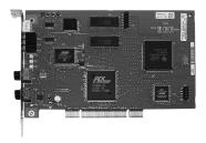
The 16-axis (1784-PM16SE) SERCOS interface card serves as a link between the SoftLogix platform and intelligent, servo drives. SERCOS is the IEC 61491 SErial Real-time COmmunication System protocol over a fiber optic medium. The SERCOS interface is an open, controller-to-digital drive interface designed for high-speed, real time, serial communications using noise-immune, fiber-optic cables.
