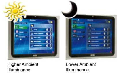
ALS is placed on the front side ,where there is an opening for light
